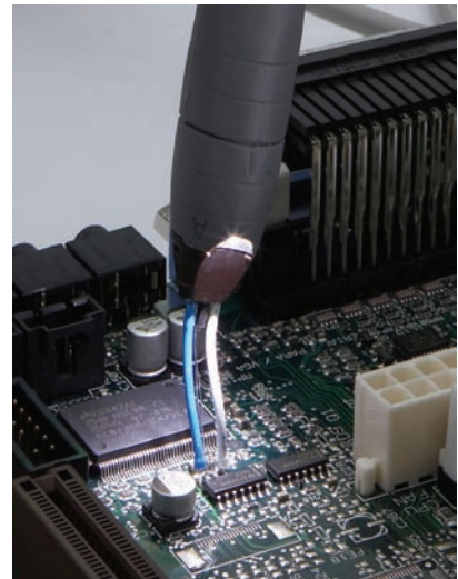
N2750A with solder-in tip
